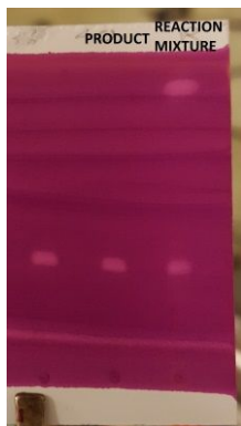
Figure S26: TLC showing the product 12 as a single polar spot with the less polar 11 at the top (on the right in a mixed spot).
